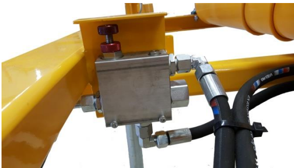
Photo I – flow control valve
