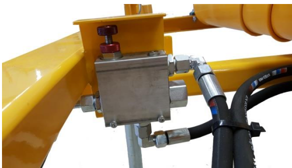
Photo I – flow control valve
